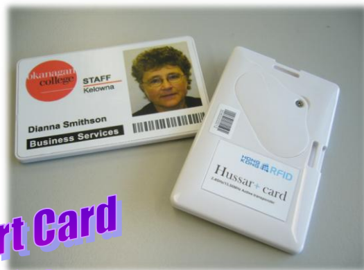
Hussar™ Card 2.4Ghz Active RFID Tag (P/N: HKRAT-CT02)
